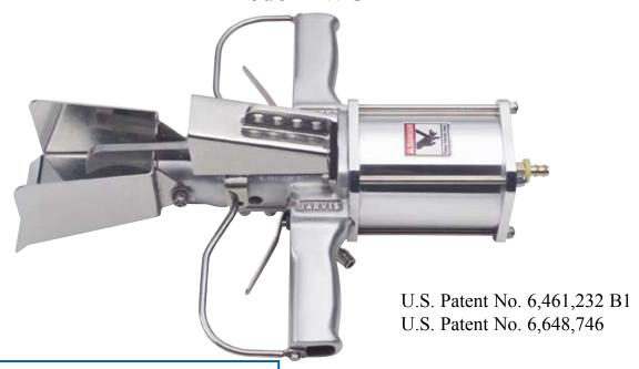
The Jarvis Model TWC-4 - pneumatically operated toe web cutter for hogs.
