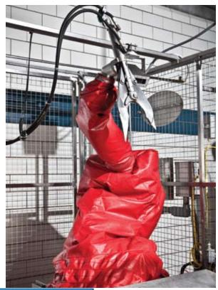
The Jarvis Model JR-50 Robotic Beef Hock Cutter for automatic hock cutting operations on the kill floor.
