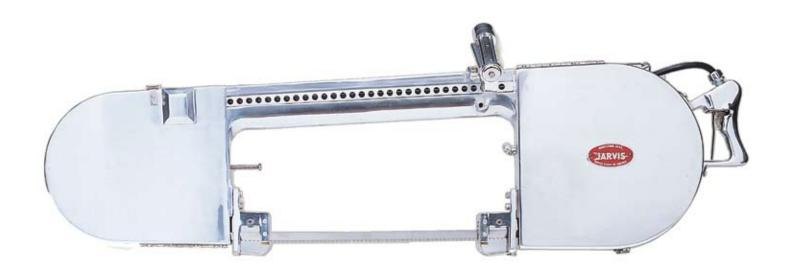
The Jarvis Model H080 - electrically powered bandsaw for high production splitting of hogs, sows or veal.
