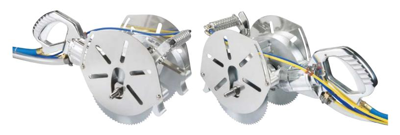
The Jarvis Model DRS-270 pneumatically powered dual-bladed ribbing saw for quick, efficient rib cutting.
